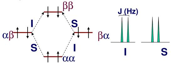
• The magnitude of the separation is called *coupling constant* (J, Hz).
