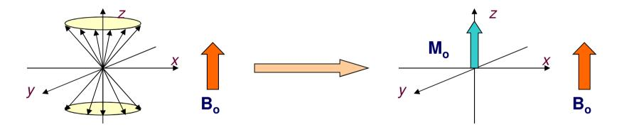
• We can decompose each little  $\mu$  in a **z** contribution and an  $\langle xy \rangle$  plane contribution. The components in the  $\langle xy \rangle$  plane are randomly distributed and cancel out. For the ones in **z**, we get a net magnetization proportional to  $N_{\alpha} - N_{\beta}$ .
