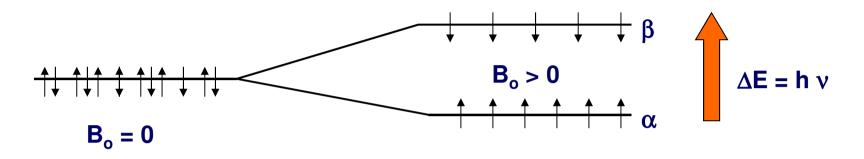
• Each level has a different *population* (*N*), and the difference between the two is related to the energy difference by the Boltzmann distribution:
