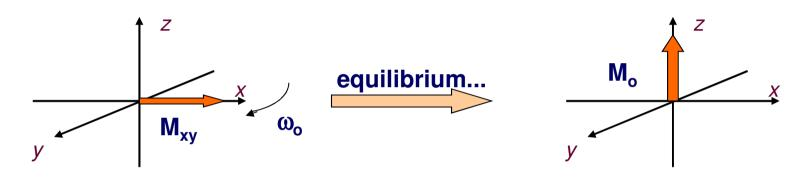
• The oscillation of  $M_{xy}$  generates a fluctuating magnetic field which can be used to generate a current in a coil:
