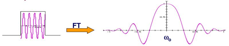
• The result is a signal centered at  $\omega_o$  which covers a wide range of frequencies in both directions. Depending on the pulse width we have wider (shorter  $t_p$ ) or narrower (longer  $t_p$ ) ranges. Remember that  $f \propto 1 / t$ .
