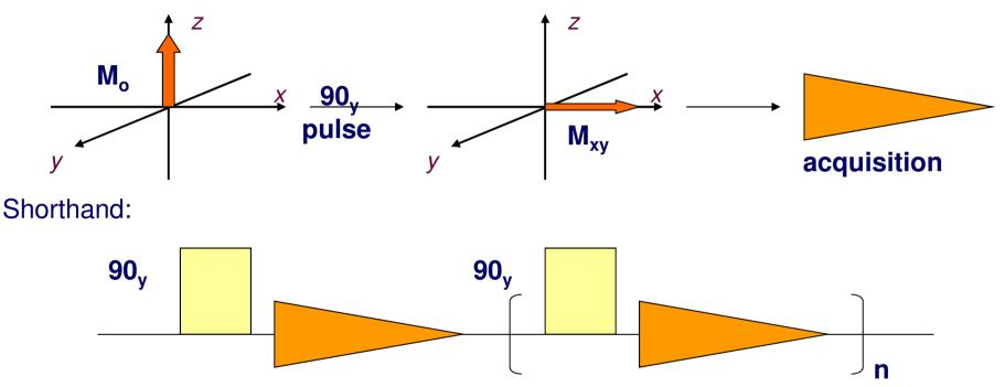
• According to the direction of the pulse, we'll use  $90_x$  or  $90_y$  (or  $90_{\phi}$  if we use other phases) to indicate the relative direction of the  $B_1$  field in the rotating frame.
