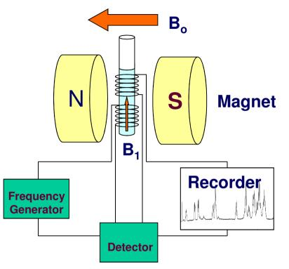
• *Magnet* - Normally superconducting. Some electromagnets and permanent magnets (EM-360, EM-390) still around.
