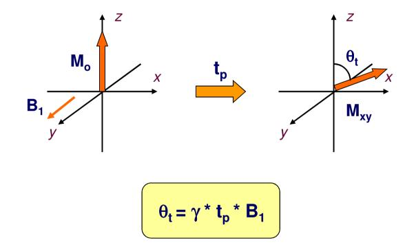
• As the pulse width for a certain flip angle will depend on the instrument ( $B_1$ ), we will therefore refer to them in terms of the rotation we want to obtain of the magnetization. Thus, we will have  $\pi / 4$ ,  $\pi / 2$ , and  $\pi$  pulses.
