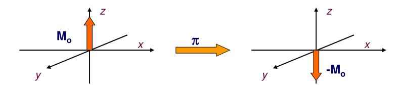
• With control of the spectrometer we can basically obtain any pulse width we want and flip angle we want.
