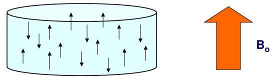
• There is always a small excess of nuclei (*population* excess) aligned with the field than pointing against it.
