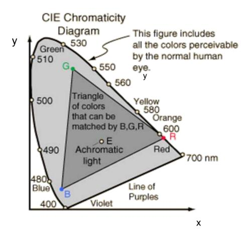
The CIE coordinates provide a device independent framework for performing color related processing
