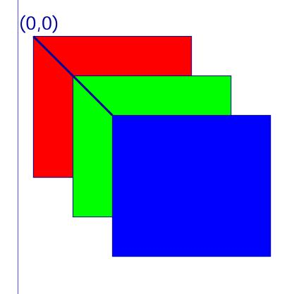
A single pixel consists of three components.
