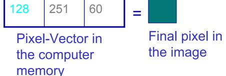
Caution! Sometimes pixels are not stored as vectors. Instead, first is stored the complete hue component, then the complete sat., then the intensity.
