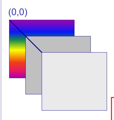
A single pixel consists of three components.
