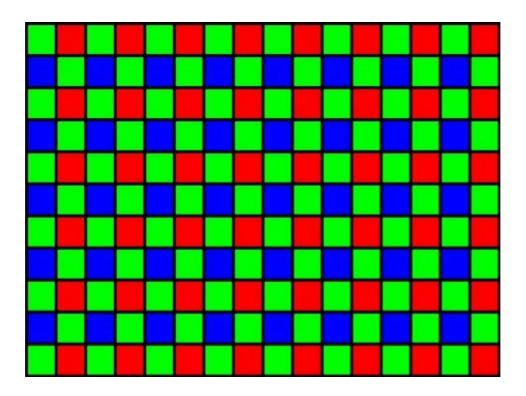
Typical sensor topology in CCD devices. The green is twice as numerous as red and blue.
