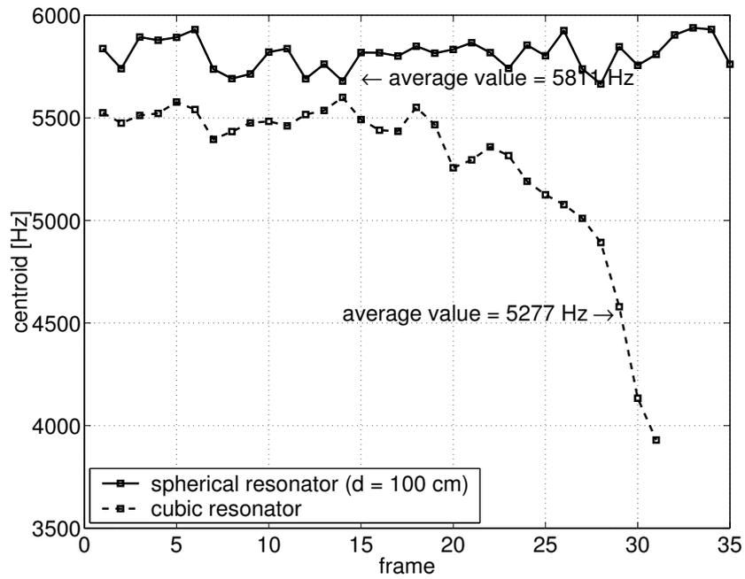
Figure 2.9: Centroids of the impulse responses of the sphere with diameter  $d = 100$  cm, volume  $= 0.5236$  m<sup>3</sup> and the cube with the same volume, represented as a function of the frame number. We can see that the sphere is brighter than the cube.
