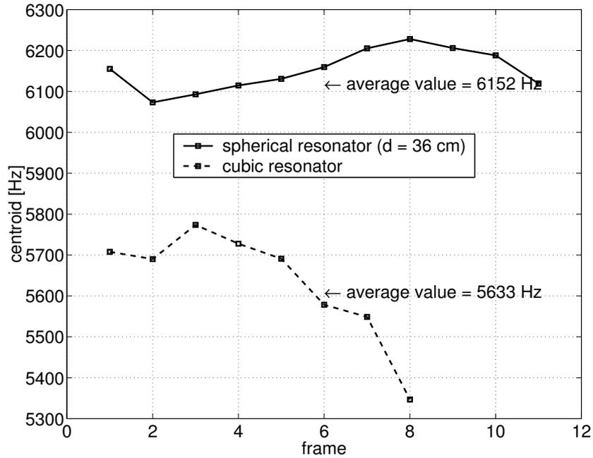
Figure 2.8: *Centroids of the impulse responses of the sphere with diameter  $d = 36$  cm, volume =  $0.0244$  m<sup>3</sup> and the cube with the same volume, represented as a function of the frame number. We can see that the sphere is brighter than the cube.*
