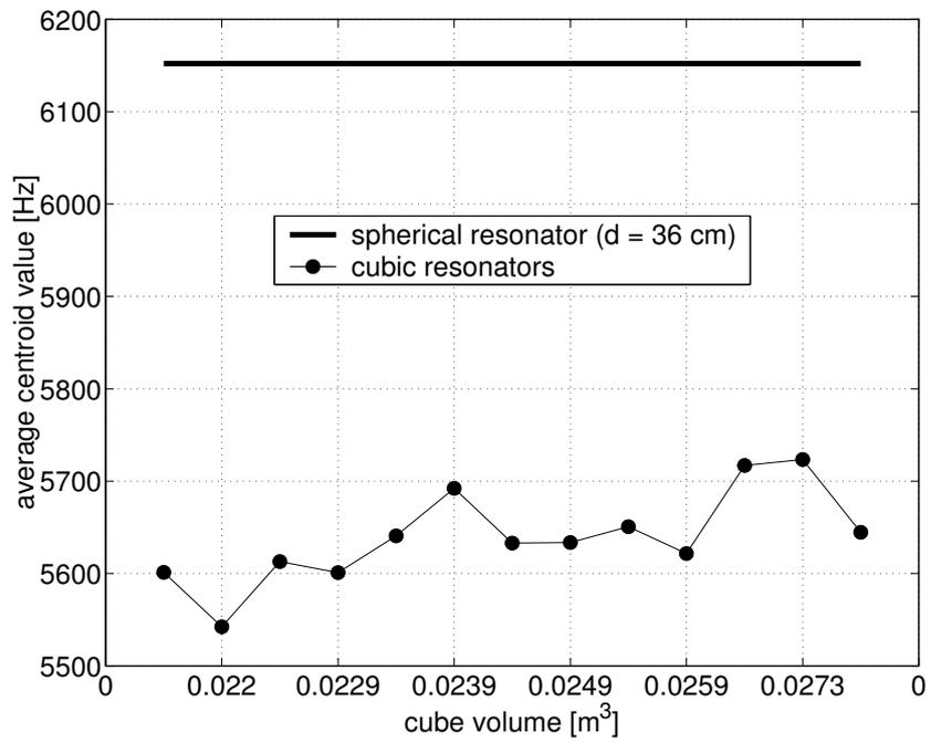
Figure 2.10: Average centroid values of the cubes in comparison with that of the sphere with diameter  $d = 36$  cm, volume =  $0.0244$  m<sup>3</sup>. We can see that the sphere is brighter than all the cubes.
