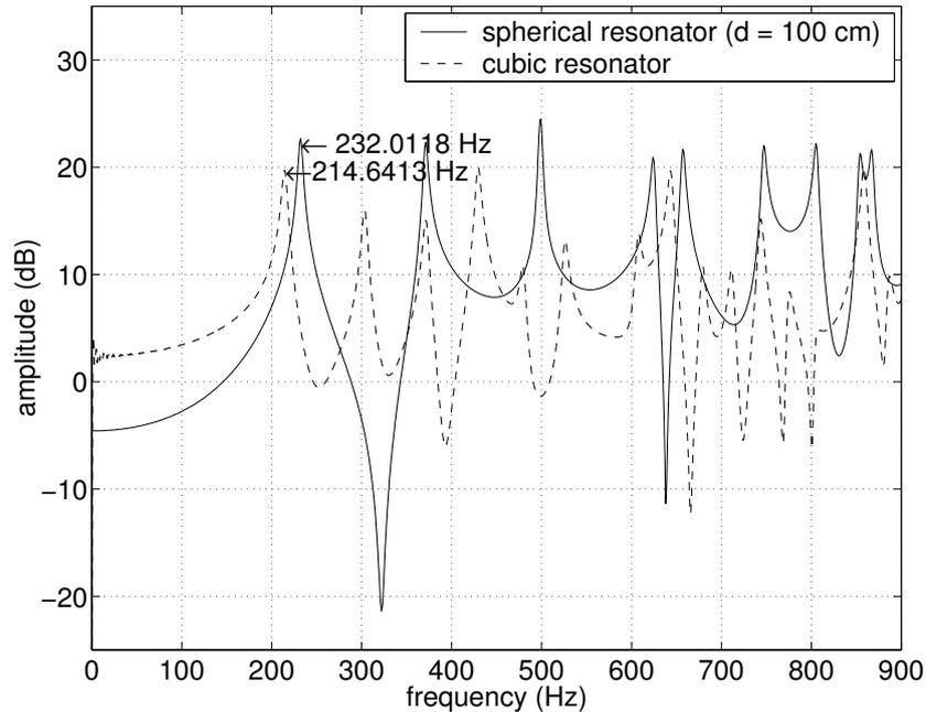
Figure 2.7: *Frequency responses, limited to the low-frequency range, of the sphere with diameter  $d = 100$  cm, volume =  $0.5236$  m<sup>3</sup> and the cube with the same volume. The first resonances of each shape are highlighted.*
