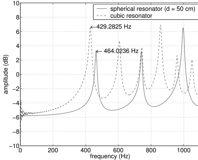
Figure 2.18: *Frequency responses, limited to the low-frequency range, of the sphere with diameter  $d = 50$  cm, volume =  $0.0654$  m<sup>3</sup> and the cube with the same volume. The first resonances of each shape are highlighted.*
