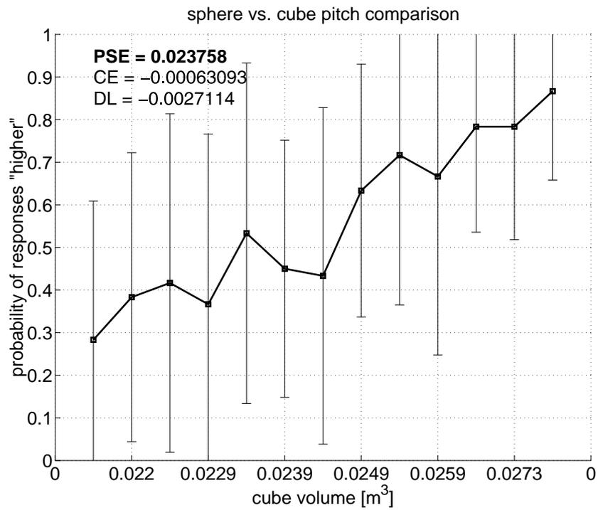
Figure 2.3: *Pitch equalization results. Second experiment. Responses probability as a function of the cubes volume and standard deviation bars. Standard stimulus: sphere with diameter  $d = 36$  cm, volume =  $0.0244$  m<sup>3</sup>.*
