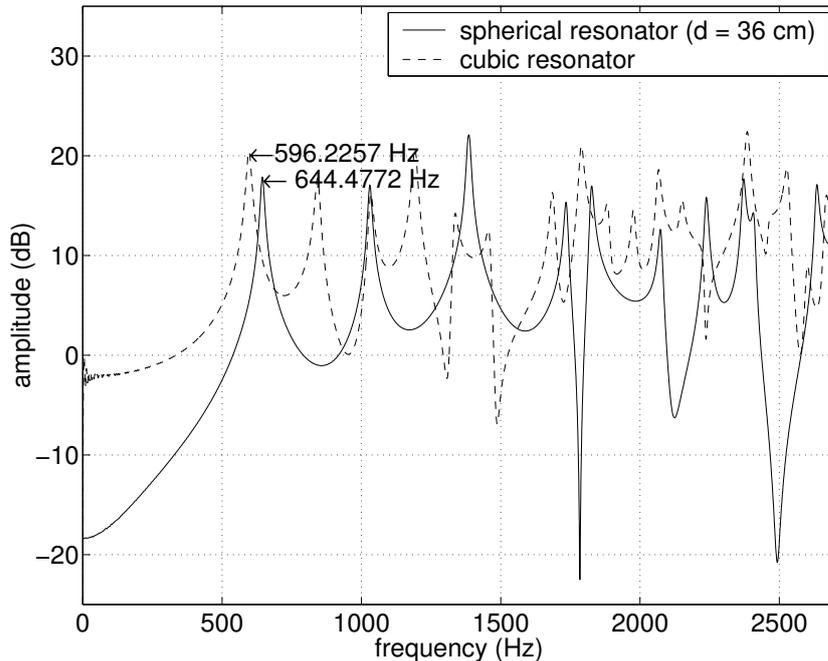
Figure 2.6: *Frequency responses, limited to the low-frequency range, of the sphere with diameter  $d = 36$  cm, volume =  $0.0244$  m<sup>3</sup> and the cube with the same volume. The first resonances of each shape are highlighted.*
