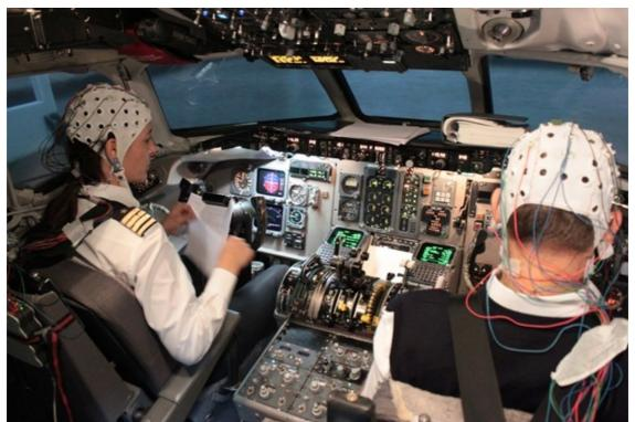
The gathering of the EEG signals in a couple of civil pilots during a simulated flight.
