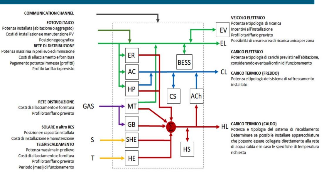
ER: Electric Resistance - AC: Air Conditioner - HP: Heat Pump - MT: Microturbine o CHP - GB: Gas Boiler - SHE: Solar Heat Exchanger - HE: Heat Exchanger - EV: Electric Vehicle - BESS: Battery Energy Storage System - ACh: Absorption Chiller -CS: Cold Storage - HS: Heat Storage
