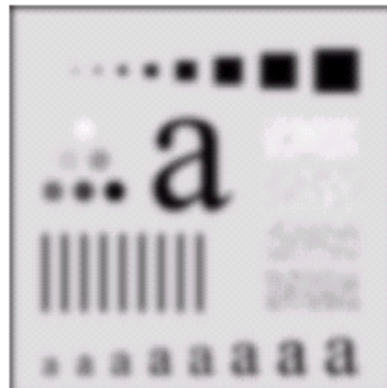
Result of filtering with Gaussian filter with cutoff radius 15
