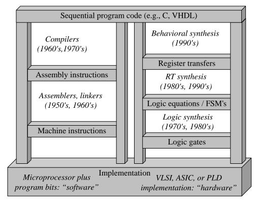
The choice of hardware versus software for a particular function is simply a tradeoff among various design metrics, like performance, power, size, NRE cost, and especially flexibility; there is no fundamental difference between what hardware or software can implement.
