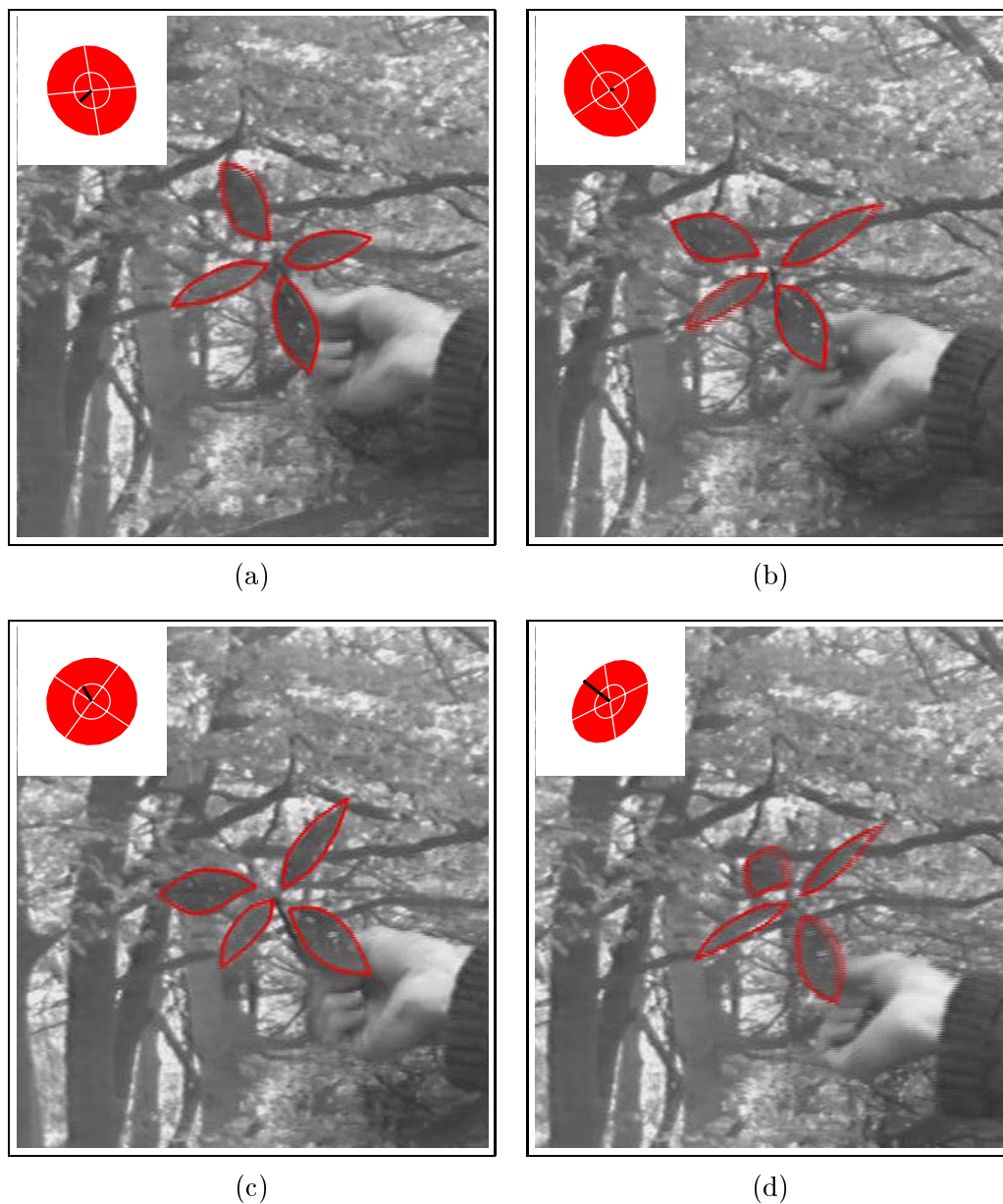
Figure 4.16: Automatic tracking is successful even against very heavy clutter. The tracked position was accurate over the entire 250 field sequence, except for a modest partial misalignment in the middle of the sequence, which lasted for 10 fields. Rendering is as in figure 4.14, and the target graphic is included to demonstrate that full 3D orientation information is being extracted.
