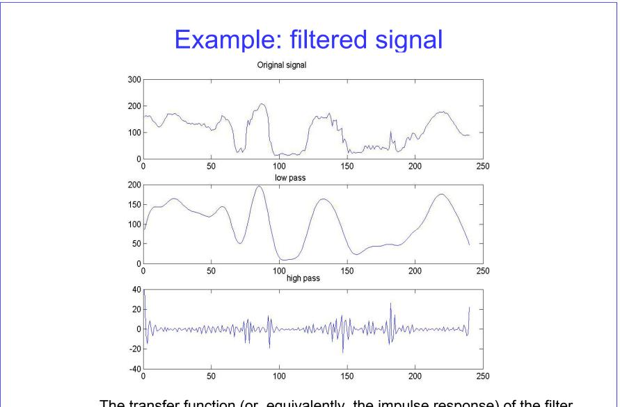
The transfer function (or, equivalently, the impulse response) of the filter determines the characteristics of the resulting signal
