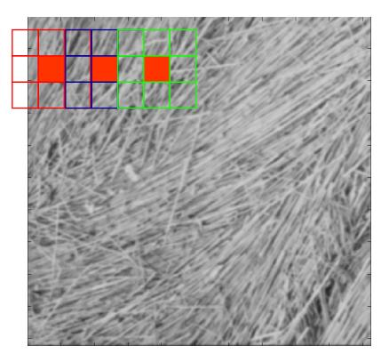
Filtering in image domain is performed by *convolving* the image with the filter kernel. This operation can be though of as a pixel-by-pixel product of the image with a *moving kernel*, followed by the sum of the pixel-wise output.
