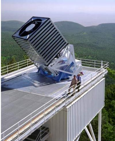
The 2.5-meter telescope at Apache Point Observatory, named the Sloan Foundation Telescope in recognition of the pivotal and generous support of the Alfred P. Sloan Foundation through all phases of the SDSS. All SDSS imaging and spectroscopy were carried out with the Sloan Telescope, equipped with a large format digital camera and fiber-fed spectrographs that measured spectra of 640 objects at a time.
