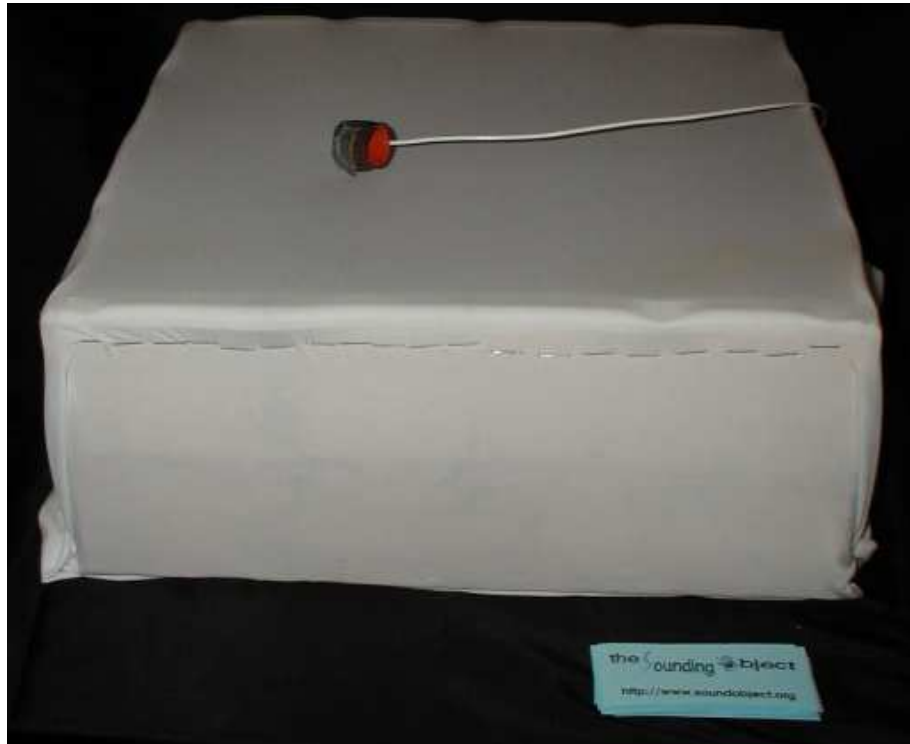
Figure 3.2: The Invisiball; the elastic cloth that can be pushed down with the sensor connected to a finger(see also figure 3.3) represents a surface where a virtual ball is rolling on.
