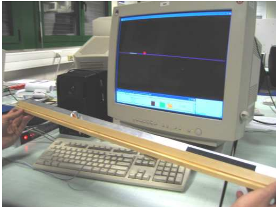
Figure 4.2: The Ballancer with the graphical spanning the whole 21" monitor (display factor 12). The photo was taken during use of the device in a game application, thus the green target area on the screen is not in the same fixed position as during the performance task described here (slightly right from the middle, according the black mark on the mechanical track). Also, the real glass marble on the track only serves demonstration purposes in the photo.
