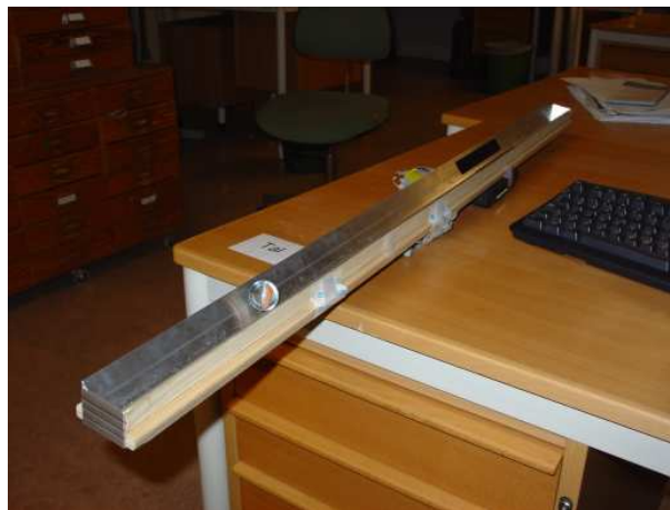
Figure 3.5: The “rolling-track” with a glass marble rolling in its upper-face aluminium track.
