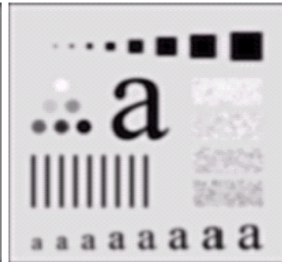
Result of filtering with Butterworth filter of order 2 and cutoff radius 30
