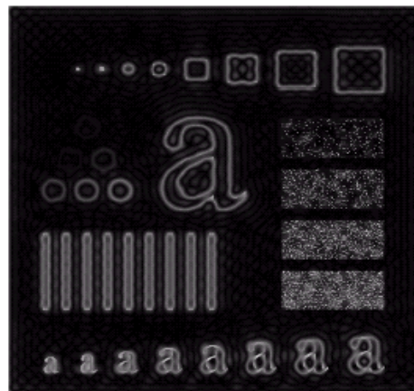
Results of ideal high pass filtering with D_0 = 30
