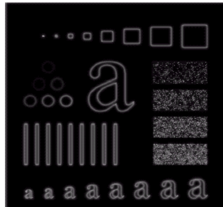
Results of Gaussian high pass filtering with D_0 = 30
