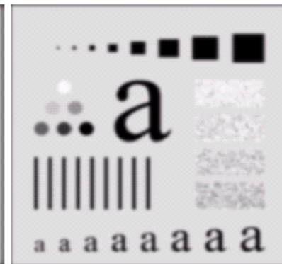
Result of filtering with Gaussian filter with cutoff radius 30
