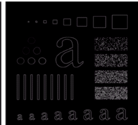
Results of Gaussian high pass filtering with D_0 = 80
