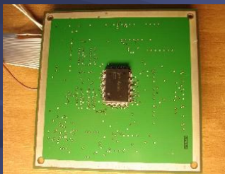
PCB with RISC IC (front)
