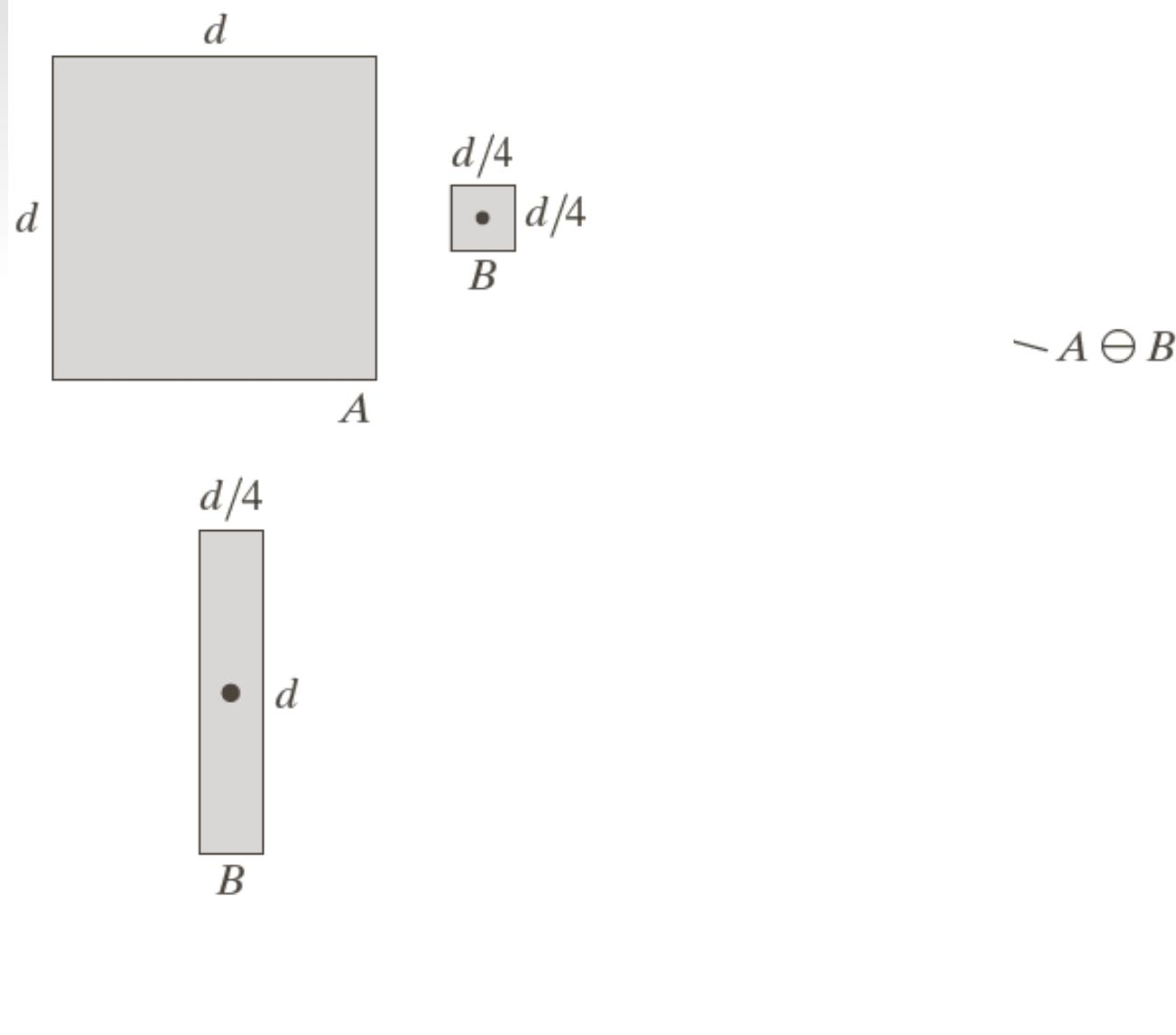
**FIGURE 9.4** (a) Set  $A$ . (b) Square structuring element,  $B$ . (c) Erosion of  $A$  by  $B$ , shown shaded. (d) Elongated structuring element. (e) Erosion of  $A$  by  $B$  using this element. The dotted border in (c) and (e) is the boundary of set  $A$ , shown only for reference.
