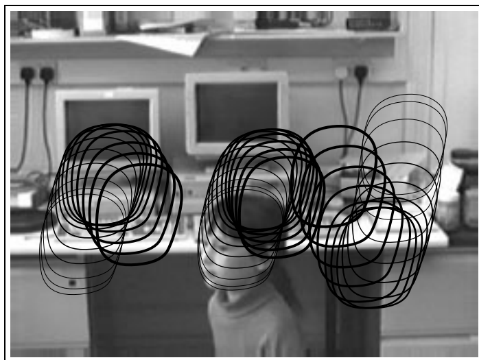
Figure 9.14: Dynamical model for a dancer. Three simulated trajectories, each of 0.84 s duration, are shown of an ARP model in a shape-space of translations. Horizontal oscillation is slow ( \beta = 0.2\text{s}^{-1} , f = 0.2\text{Hz} ) and broadly distributed ( \bar{\rho} = 300 pixels), representing the motion of the dancer to and fro, across the room. Vertical oscillation is faster ( \beta = 0.5\text{s}^{-1} , f = 1\text{Hz} ) and more tightly distributed ( \bar{\rho} = 100 pixels), representing the bobbing motion of the head.
