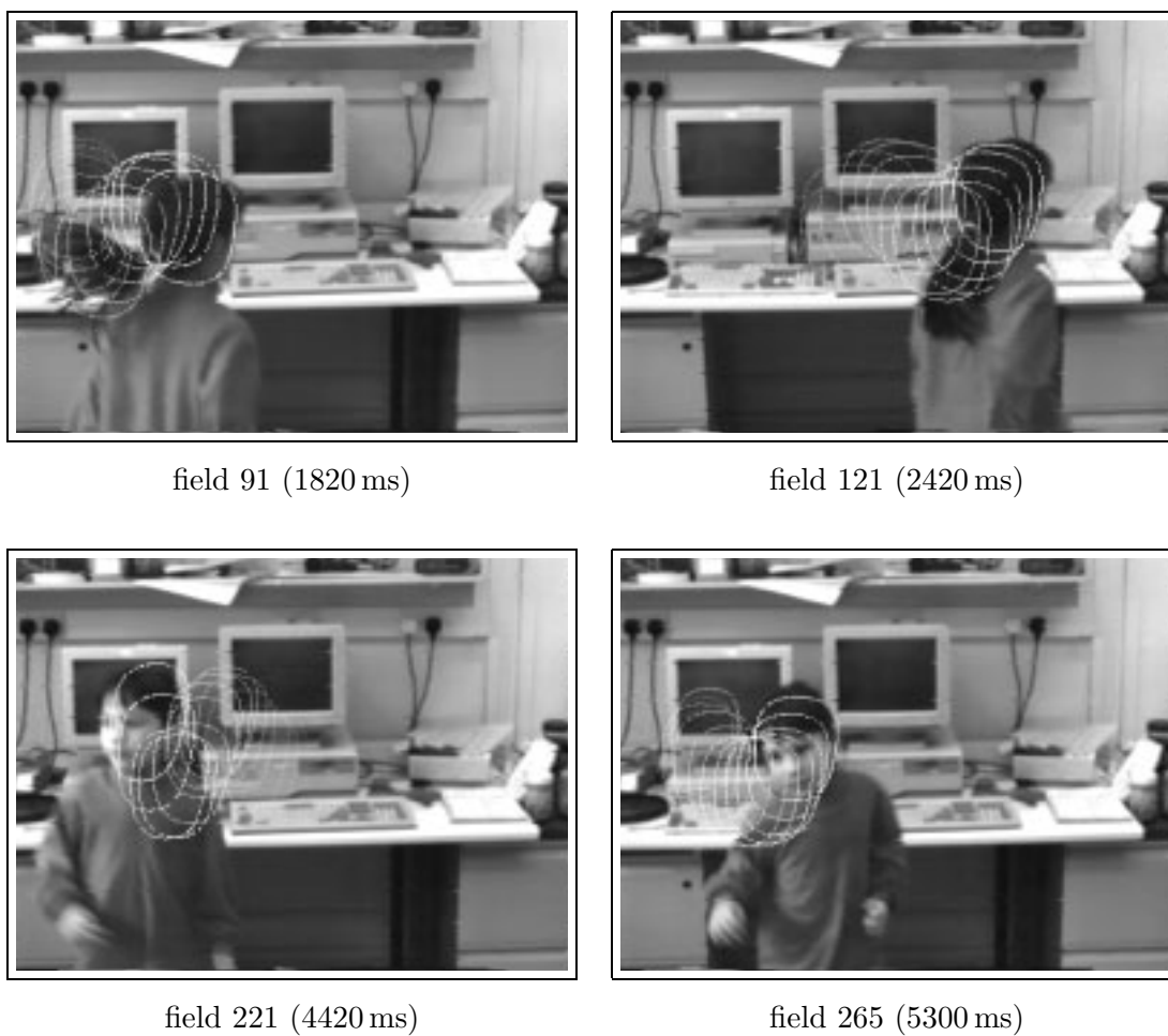
Figure 12.11: Tracking agile motion in clutter. The test sequence consists of 500 fields (10 seconds) of agile dance against a cluttered background. The dancer's head is tracked through the sequence. Several representative fields are shown here, each with a trail of successive mean tracked head positions at intervals of 40 ms. The CONDENSATION algorithm used N = 100 samples per time-step to obtain these results.
