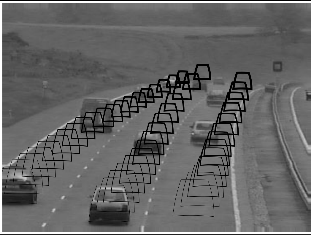
Figure 9.13: Dynamical model for traffic. Three simulated trajectories for an ARP set up to represent the traffic pattern, each initialised with a velocity in shape-space corresponding to translation along the road, coupled with shrinkage consistent with perspective scaling. Translational parameters are \beta = f = 0 (constant-velocity) with \gamma_0 = 35 \text{ pixel.s}^{-3/2} , allowing the paths to veer over longer times. Affine deformations are critically damped ( f = 0 ) with a long time-constant ( 1/\beta = 10 \text{ s} ), and largely deterministic ( \bar{p} = 2 \text{ pixels} ), allowing the outline to shrink steadily. Contours are plotted here at intervals of 200 ms.
