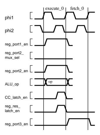
Figure 7-29. Execution of register/register operations.
