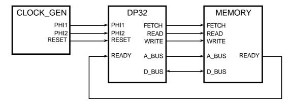
Figure 7-10. Test bench circuit for DP32.
