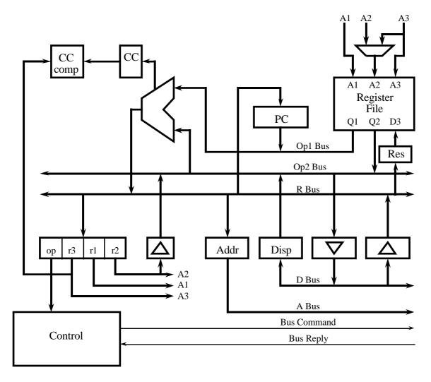
Figure 7-16. DP32 data paths block diagram.
