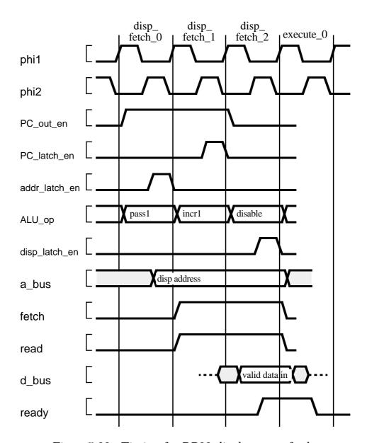
Figure 7-28. Timing for DP32 displacement fetch.
