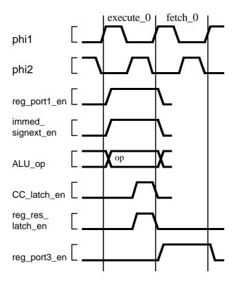
Figure 7-30. Execution of register/immed operations.
