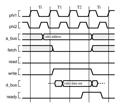
Figure 7-5. DP32 bus write transaction.
