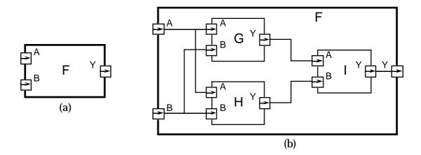
Figure 1-1. Example of a structural description.
