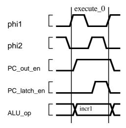
Figure 7-32. Execution of branch with branch not taken.
