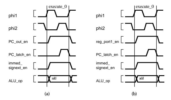
Figure 7-31. Execution of quick branch with branch taken.
