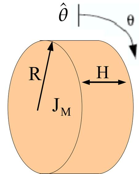
$$\begin{aligned} \mathbf{I}_J &= \int_0^H \int_0^R r^2 dm = \int_0^H \int_0^R \rho r^2 dV = \\ &= \rho \int_0^H \int_0^R r^2 (2\pi r) dr dh = (2\pi\rho) \int_0^H dh \int_0^R r^3 dr \\ &= (2\pi\rho) \int_0^H dh \left[ \frac{r^4}{4} \right]_{0,R} = 2\pi \frac{M}{(\pi R^2 H)} \frac{R^4}{4} H \\ &= \frac{1}{2} MR^2 \end{aligned}$$
